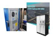
The BYD containerized Energy Storage System is rated at 250 kW (300 KVa) and 500 KWh with nominal output voltage of 415 VAC at a frequency of 50Hz and is outfitted with environmental controls, inverters and transformers, all self-contained, in a 40 foot shipping container to provide stable power supply.
