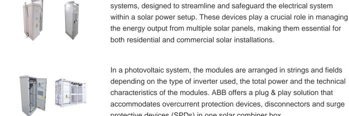
In a photovoltaic system, the modules are arranged in strings and fields depending on the type of inverter used, the total power and the technical characteristics of the modules. ABB offers a plug & play solution that accommodates overcurrent protection devices, disconnectors and surge protective devices (SPDs) in one solar combiner box.
