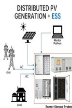
What are energy storage technologies? Energy storage technologies are segmented into those that can deliver precise amounts of electricity very rapidly for a short duration (capacitors, batteries and flywheels), as well as those that take longer to ramp up, but can supply tens or hundreds of megawatts for many hours (compressed air energy storage and pumped-storage hydropower).
