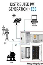
What are energy storage systems? Energy storage systems allow energy consumption to be separated in time from the production of energy, whether it be electrical or thermal energy. The storing of electricity typically occurs in chemical (e.g., lead acid batteries or lithium-ion batteries, to name just two of the best known) or mechanical means (e.g., pumped hydro storage).
