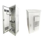
100kWh 200kWh Outdoor Cabinet Type Energy Storage System. The outdoor cabinet energy storage system, is a compact and flexible ESS specifically designed for small C& I loads. Rated Charge/Discharge Power: 60kW: Rated Grid Voltage: AC400V: Grid Voltage Range-15%~+ 15%: Rated Grid Frequency: 50Hz: Frequency Range: 5Hz: Rated Current: 86A
