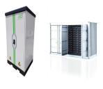
How many batteries can be stored in the evervolt energy storage system? The EverVolt energy storage system comprises of modular batteries to meet varying customer needs. Each battery module weighs about 55lbs each enclosed in a battery cabinet to ensure easy installation. The battery cabinet can house up to a maximum of 6 batteries with a usable storage capacity of 17.1 kWh.
