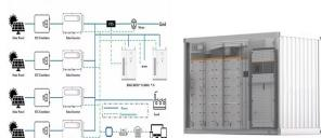
A hybrid energy storage system combined with thermal power plants applied in Shanxi province, China. Taking a thermal power plant as an example, a hybrid energy storage system is composed of 5 MW/5 MWh lithium battery and 2 MW/0.4 MWh flywheel energy storage based on two 350 MW circulating fluidized bed coal-fired units.
