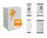
Comprehensive energy storage solutions with modular design, high-performance lithium iron phosphate batteries, and advanced management systems. 2 rows and 2 clusters, 2P240S, including 21 51.2V/280Ah battery PACK, 2 battery high voltage boxes, total battery capacity 300KWh: 1: set: 3: Energy storage converter: 150KW, off-grid and on-grid
