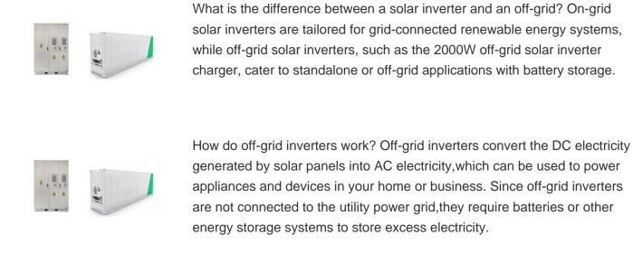
Do on-grid inverters provide backup power if the power grid goes down? However,on-grid inverters do not provide backup powerin the event of a power outage. When the utility power grid goes down,your solar power system will also be shut down for safety reasons. Off-grid inverters,also known as standalone inverters,are designed to work independently of the utility power grid.
