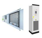
The CLC20-1000 is an energy storage container with air cooling. A modular compact battery rack is paired with independent air ducts and specialized industrial air conditioning. Special lithium iron phosphate battery cells and high-safety battery modules are also included in the system.
