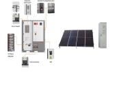
Types of Grid Connected PV Systems. String Inverter System: This is the most common type of grid-connected PV system. It uses a string inverter to convert DC electricity from the solar panels to AC electricity ???
