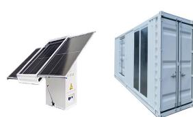
While having a high energy density and fast response time, the systems also convince by a design life of 20 years, or 7,300 operating cycles due to a very low degradation level. The NAS battery storage solution is containerised: each 20-ft container combines six modules adding up to 250kW output and 1,450kWh energy storage capacity.
