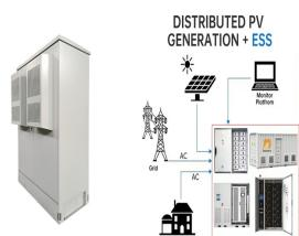
To facilitate the future installation of battery storage systems, newly constructed single-family buildings with one or two dwelling units are required to be energy storage ready. An energy storage system is defined in the 2022 Energy Code as one or more devices assembled together to store electrical energy and supply electrical energy to
