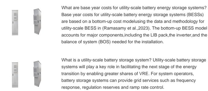
What is a battery energy storage system? A battery energy storage system (BESS) is an electrochemical device that charges (or collects energy) from the grid or a power plant and then discharges that energy at a later time to provide electricity or other grid services when needed.
