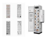
Product Introduction. Huijue Group's Industrial and commercial energy storage system adopts an integrated design concept, integrating batteries, battery management system BMS, energy management system EMS, modular converter PCS and fire protection system into one cabinet. Modular design allows for flexible capacity expansion and adapts to a variety of application ???
