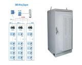
Suitable for solar inverters with 2 independent MPPT trackers, 2ways in, 2ways output. Matches the Conversol Max 8kW, 11kW, and all the inverters with dual input. SPD, fuse terminals, DC isolator, IP65 box. Why do I need a combiner box? First of all for protecting the installer and later the users. During the installation of solar panels or when maintenance is required, the strings ???
