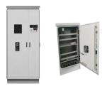
The role of the combiner box is to bring the output of several solar strings together. Daniel Sherwood, director of product management at SolarBOS, explained that each string conductor lands on a fuse terminal and the output of the fused inputs are combined onto a single conductor that connects the box to the inverter."This is a combiner box at its most basic, ???
