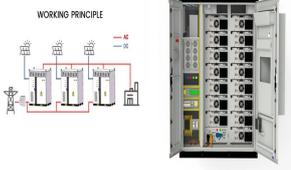
This Hybrid Solar Air Conditioner uses solar panel energy or grid power or combination of solar panel energy and grid power. Its first priority is always solar energy. If there is not enough solar ???
