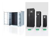
What is a 15kW transformerless grid tie inverter? 15kW transformerless grid tie inverter for three phase on grid solar power system, which converts 200-820V wide DC input voltage to 208V/240V/380V AC output voltage feed the power into the grid. LCD display, can set main general parameters. Multiple grid tie inverters can be operated in parallel.
