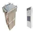
CEMLINE Flash Tanks are used to flash steam from high temperature condensate prior to introducing into low pressure lines and to flash condensate prior to returning to the boiler or condensate tank. CEMLINE Flash Tanks are ASME code constructed and stamped for 150 PSI working pressure of carbon steel and have a prime painted exterior. [???]
